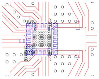
We recommend that all N/C pins be grounded and sufficient number of vias to be present under the ground plane to insure good RF and thermal grounding. Pins 13 and 18 are connected to the RFout trace.
